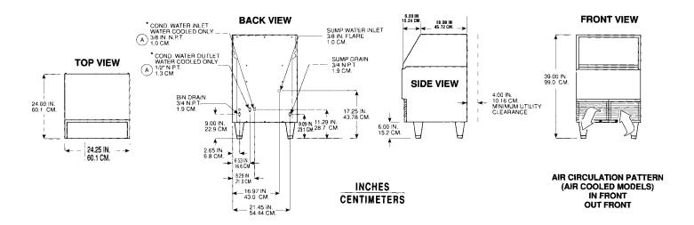
INSTALLATION NOTE: Allow 6" minimum space at back for utility connections.
