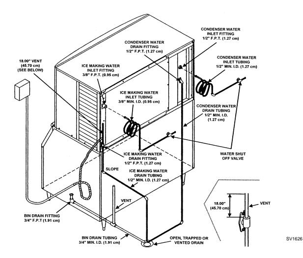
**Typical Water Supply Drain Installation**
