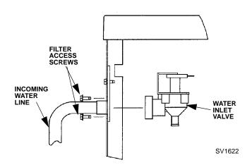
**Water Inlet Valve Removal**
