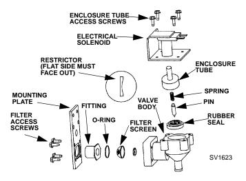
**Exploded View of Water Inlet Valve**
