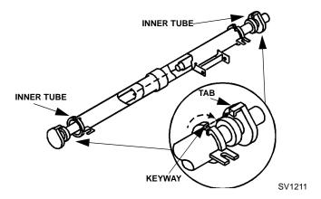
**Water Distribution Tube Disassembly**
