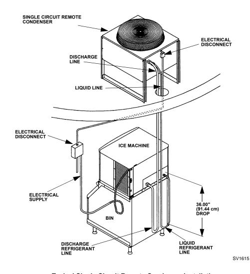
**Typical Single Circuit Remote Condenser Installation**
