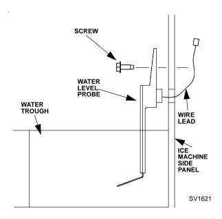
**Water Level Probe Removal**
