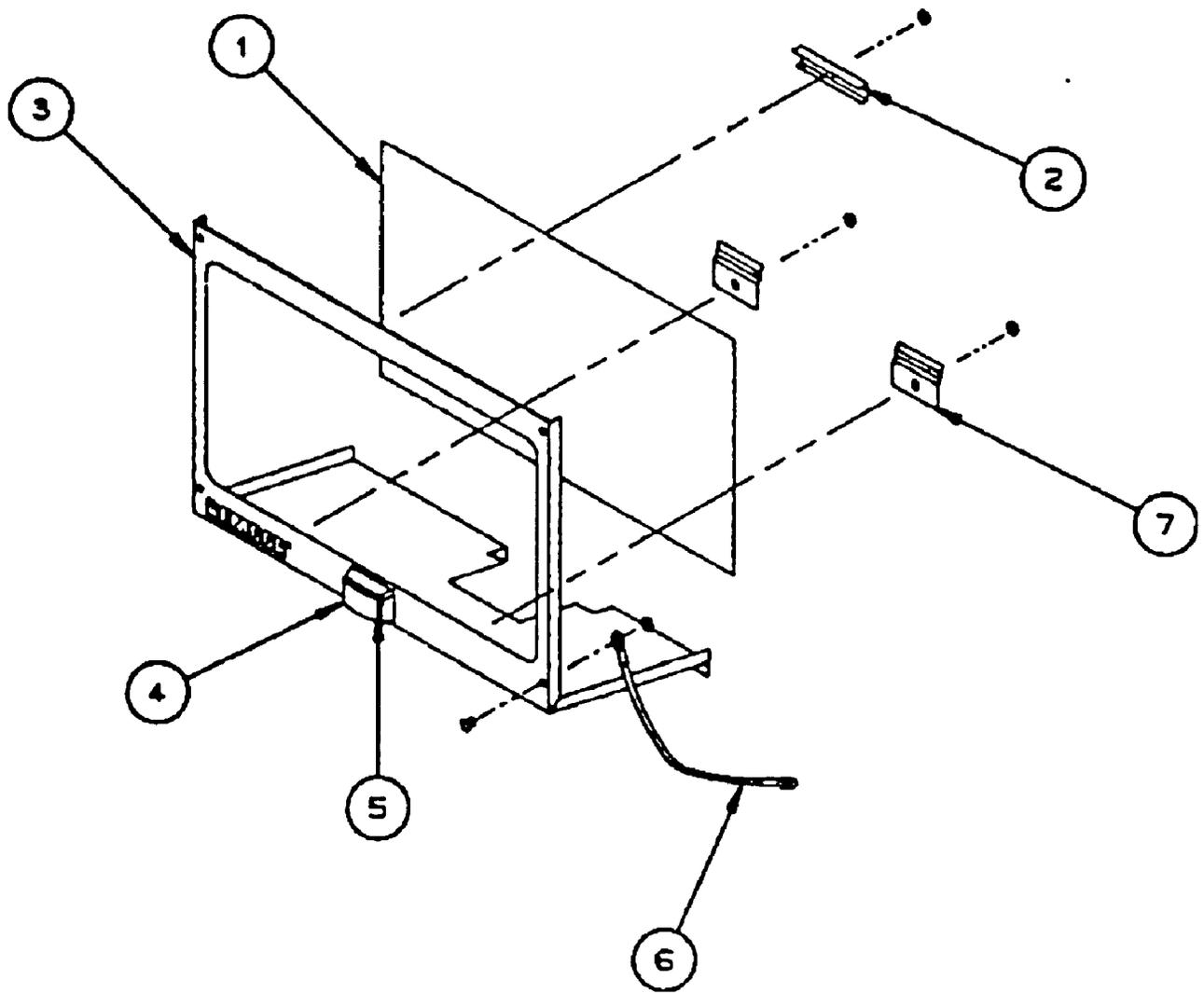
**FIGURE 14. EXPLODED VIEW & PARTS LIST DB90-BC MERCHANDISER SECTION**
