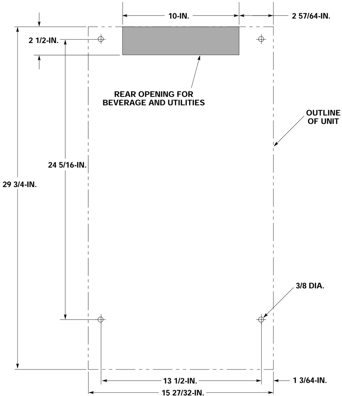
**NOTE:** 1) Shaded areas indicate openings in cabinet bottom needed for utilities and beverage tubing.
