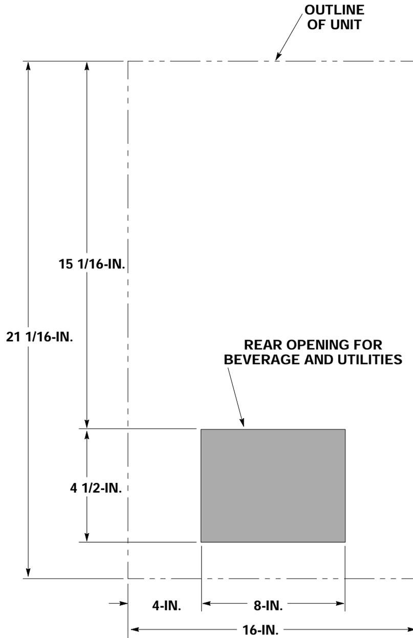
**NOTE:** 1) Shaded areas indicate openings in cabinet bottom needed for utilities and beverage tubing.
