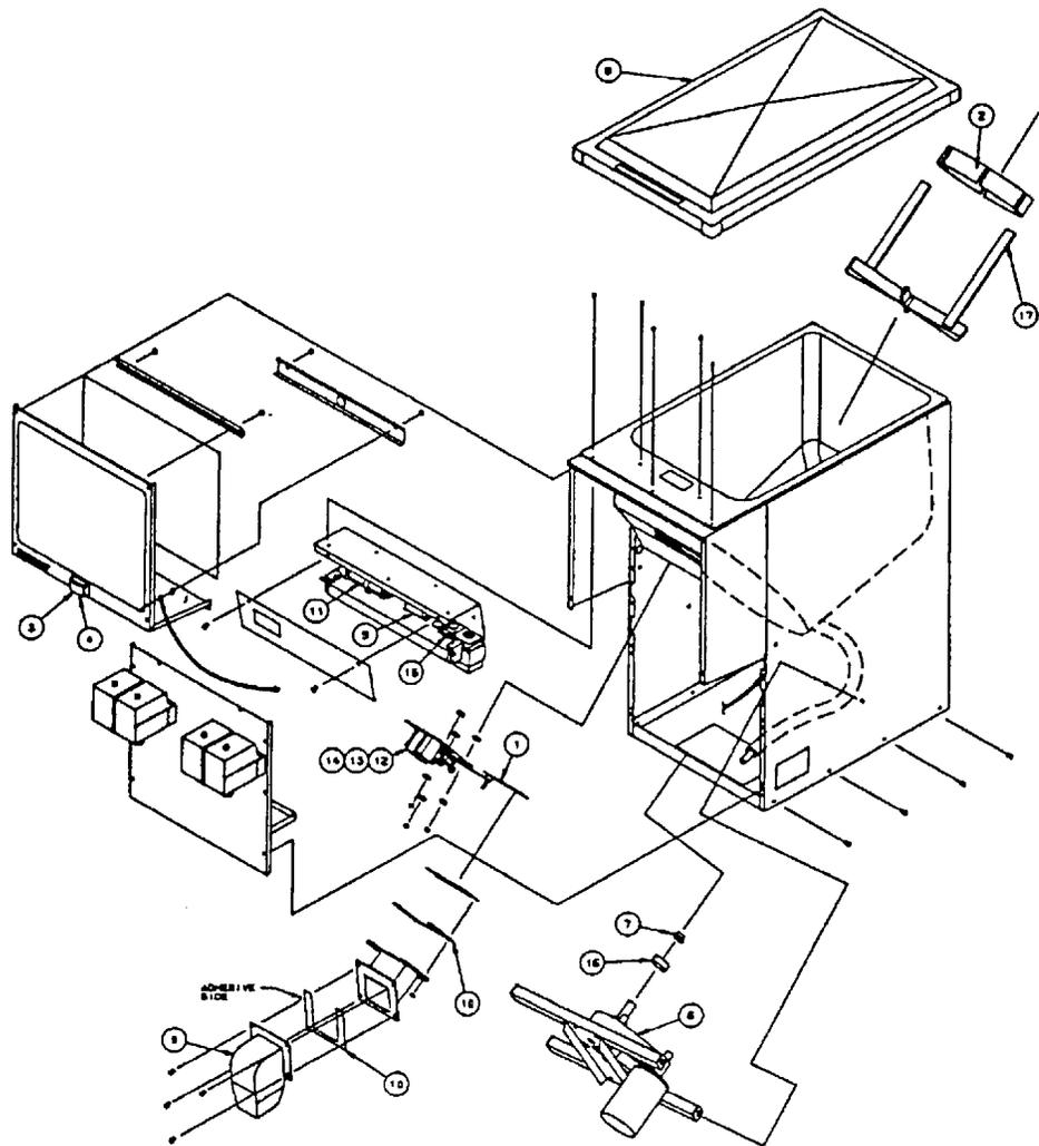
**FIGURE 13. EXPLODED VIEW & PART LIST DB90-BZ (NO SINK)**
