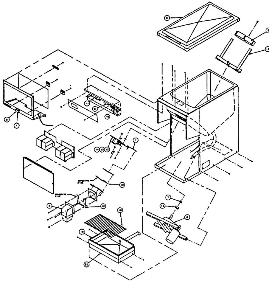
**FIGURE 12. EXPLODED VIEW & PART LIST DB90-B**
