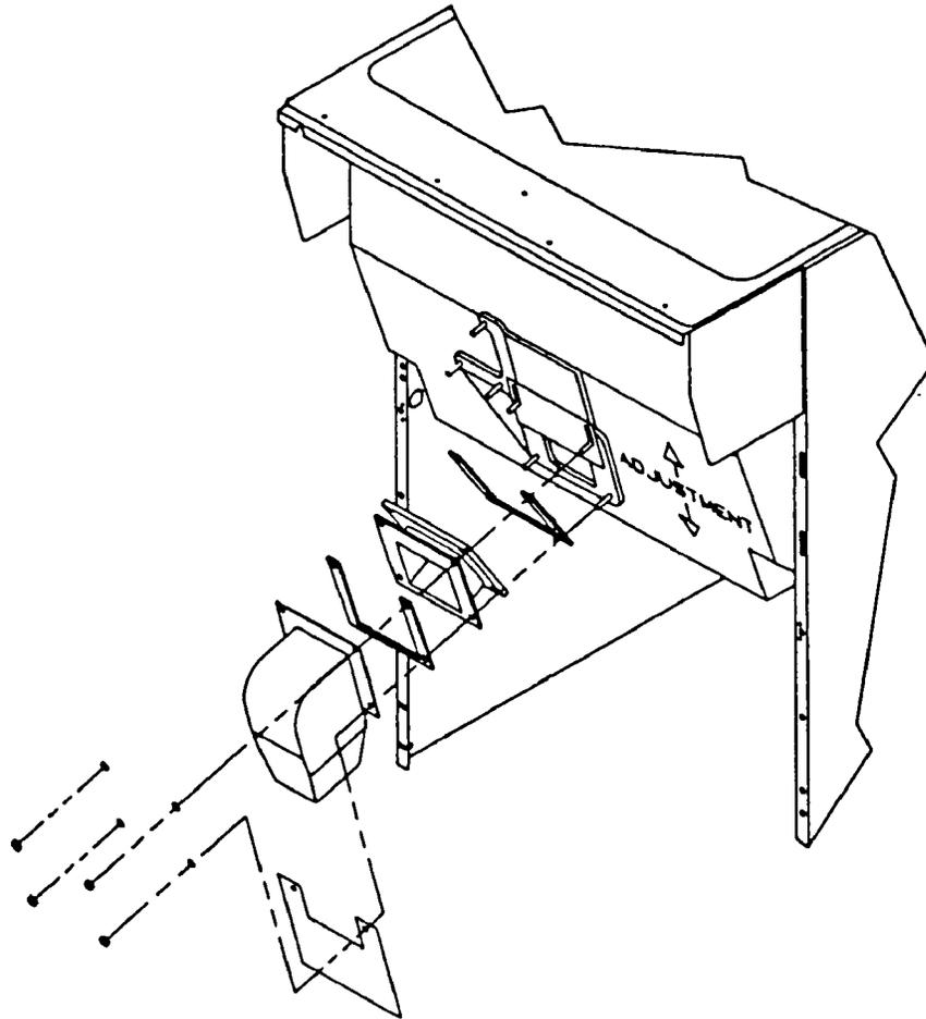
**FIGURE 2. GATE RESTRICTOR PLATE**
