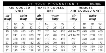
†Production for Dice and Half Dice cubes. Regular cube is 7% less than chart and kWh/100 lbs. increases 7%.
