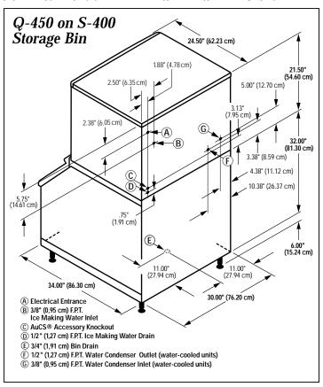
**Installation Note** - Minimum Installation Clearance: Top/Sides are 8" (20.32 cm), Back is 5" (12.7 cm).
